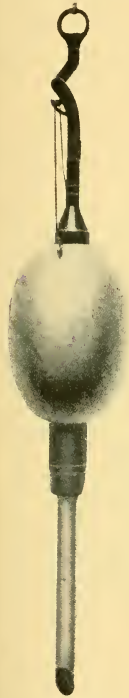
FIG. 6.—SIGSBEE'S SOUNDING-TUBE. (From Brennecke.)
